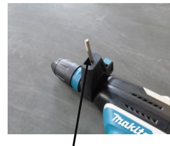
Foam allows for bolt to stay in place.
